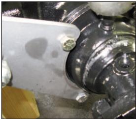
Install the master cylinder bracket to the flange of the universal joint ball with two 3/8-24x1-3/4" thin head bolts provided. Install the Master Cylinder on the bracket using two 5/16-24 x 1-1/2" bolts and nuts. Use Loctite on the threads of all bolts.
