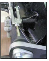
to act as a locking nut. Pull the pedal up and adjust the master cylinder rod so there is a slight bit of play on the clevis pin.
