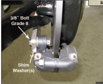
When you have your spacing worked out, use Loctite 242 Threadlocker on these bolts/nuts. Torque the 3/8-24 Grade 8 bolts to 40 ft.lbs.
