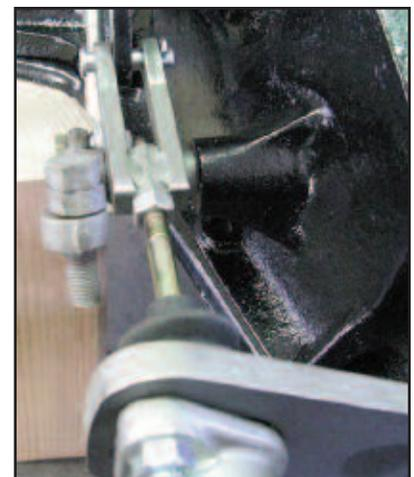
DO NOT use the shim wahers with the standard Ford universal ball cap or any other application where the mating surface does not have a machined recess.
