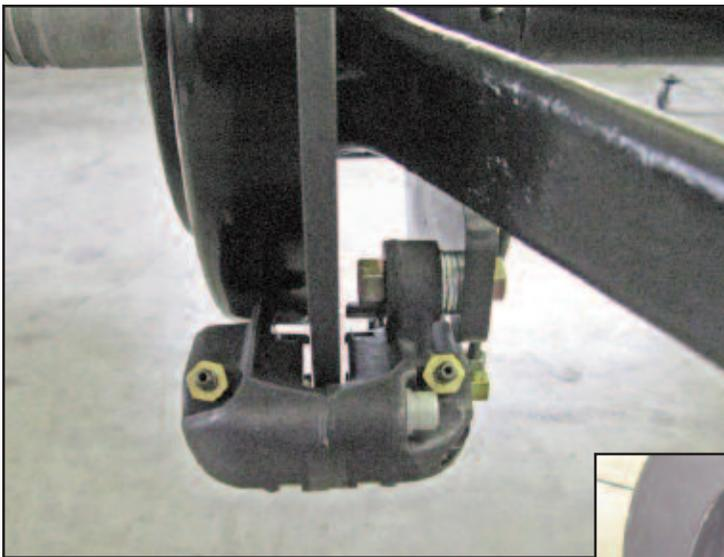
When you have your spacing worked out, use Loctite 242 Threadlocker on these bolts/nuts. Torque to 40 ft/lbs.
