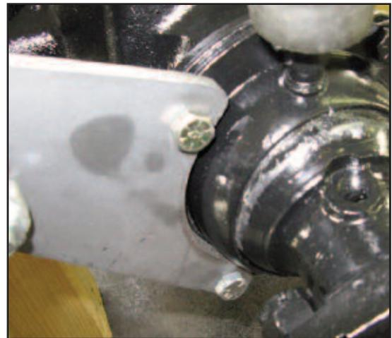
8. Install the master cylinder bracket to the flange of the universal joint ball with two 3/8-24x1-3/4" thin head bolts provided. Install the Master Cylinder on the bracket using two 5/16-24 x 1-1/2" bolts and nuts. Use Loctite on the threads of all bolts.
