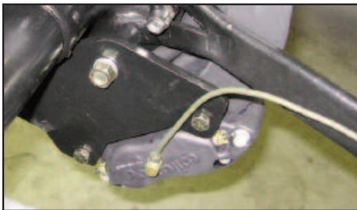
12. Install metal brake lines, bending by hand to follow radius rod as per picture. Secure the steel brake lines to the radius rods with the Zip ties provided.
