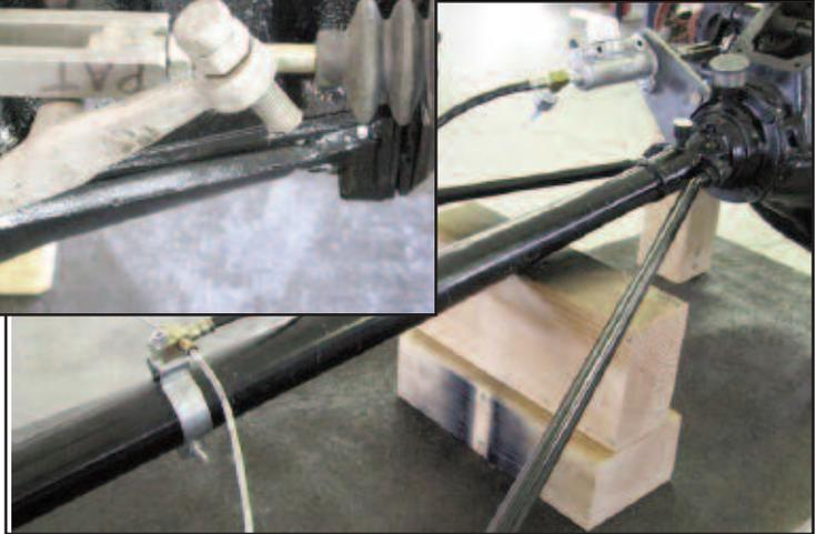
11. Install the pressure line clamp on your torque tube approximately 21" in front of the back flange of the torque tube. It can be installed on the top or bottom of the tube, whatever you need on your car.
