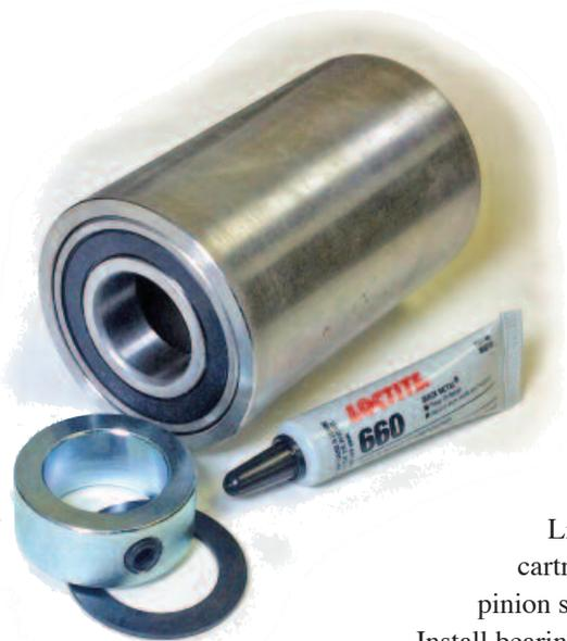
1. Try your drive shaft through the bearing cartridge. You may need to dress the shaft with a file particularly the area just in front of the pinion gear to relieve any swelling of the shaft. You may also need to dress the driveshaft with fine emery paper to get the bearing cartridge to fit properly. The hardened inner race of the bearing will not tolerate irregularities in the surface of the drive shaft..
