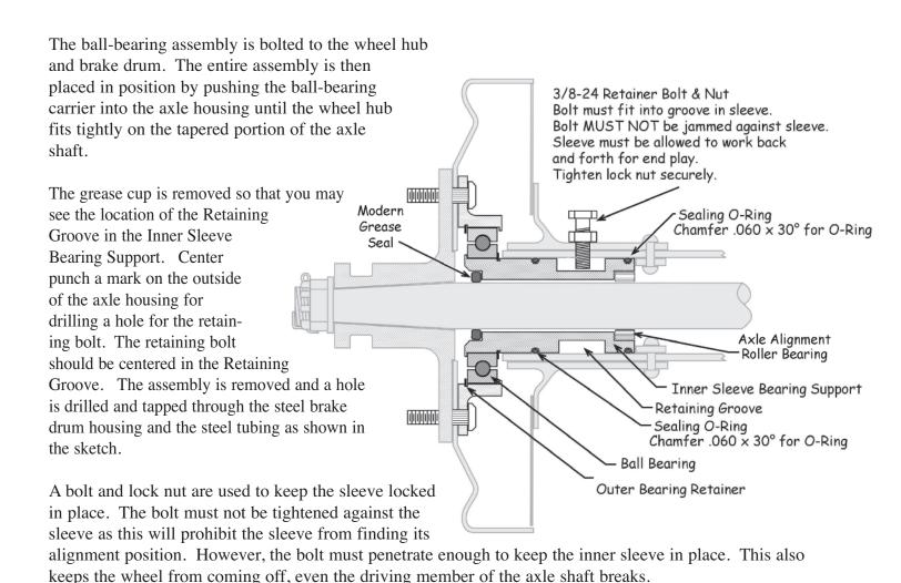
The steel inner sleeve or bearing support has a hole of sufficient diameter to clear the axle by 1/8 inch. The outer diameter of the bearing support has very close tolerance to the inside diameter of the steel tubing to eliminate transfer of bending strains to the axle. The ball-bearing is held in place by the steel outer bearing retainer
