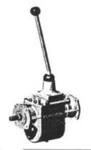
The original Warford transmission was an auxiliary unit that replaced 12" of the drive shaft at the rear of the engine. Four additional forward speeds and two reverse speeds are added and offer a true neutral.
