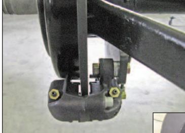
When you have your spacing worked out, use Loctite 242 Threadlocker on these bolts/nuts. Torque to 40 ft/lbs.
