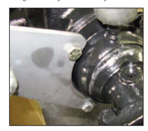
8. Install the master cylinder bracket to the flange of the universal joint ball with two 3/8-24x1-3/4" thin head bolts provided. Install the Master Cylinder on the bracket using two 5/16-24 x 1-1/2" bolts and nuts. Use Loctite on the threads of all bolts.
