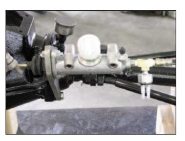
**Note:** We have found that it is difficult to get a good seal at the O-ring connection on both the Master Cylinder Cap installed in Step 13 and the Fluid Reservoir installed in step 14.
