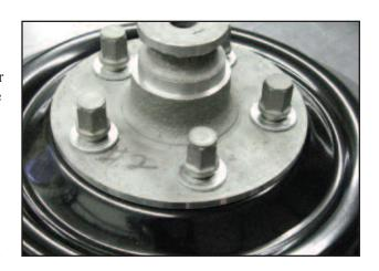
assembly, your existing wheel hub, and the 3/8" spacer plate provided in this kit.) Install the new disc brake drum on your original hubs using lug nuts and large washers. Tighten in sequence so as to pull the hub tight against the drum evenly. Be careful not to burr the lug bolt shafts.
