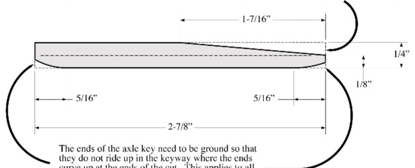
The ends of the axle key need to be ground so that they do not ride up in the keyway where the ends curve up at the ends of the cut. This applies to all axle keys on all Model T axles.
